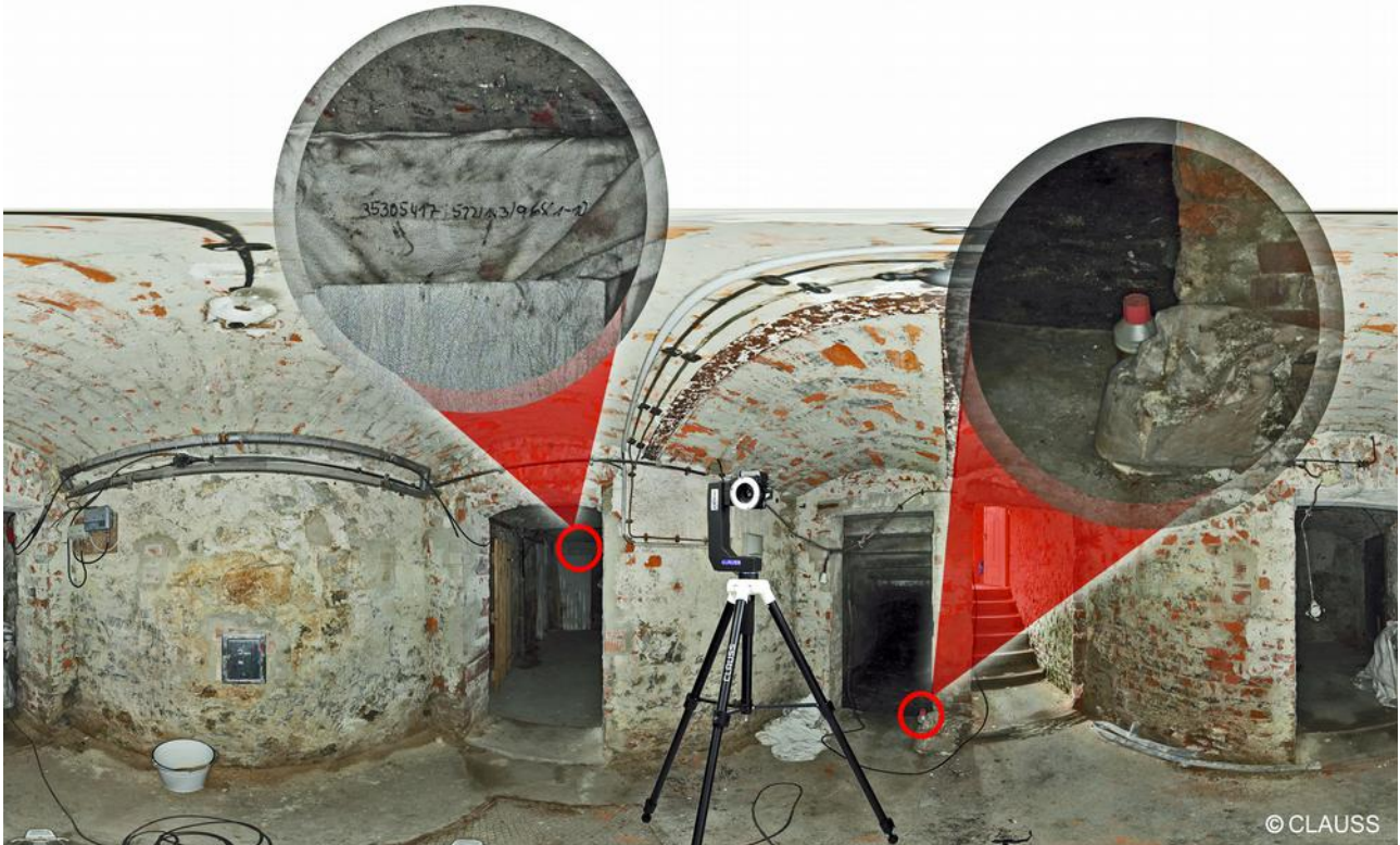
Fig. 2: Crime scene documentation with piXplorer CSD model. In all cases, an additional heavy duty tripod has to be used, see picture.
